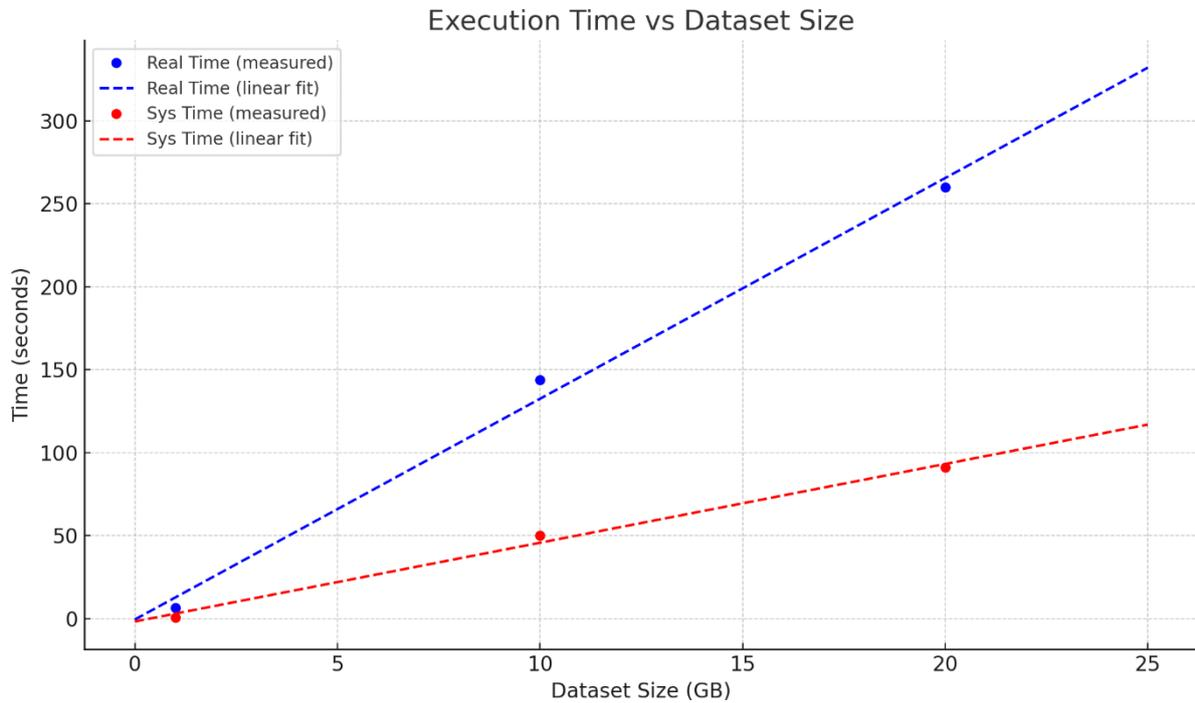
This chart, an extrapolation of the dataset execution time test results, demonstrates how real and sys execution times scale with dataset size:
